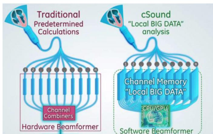
**Figure 4:** Hardware vs. Software Beamformer
